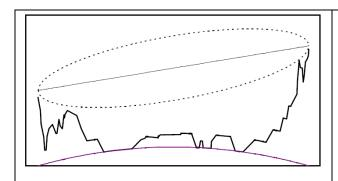
No obstruction loss (0 dB) if the propagation is open LOS with clearance over the whole path
